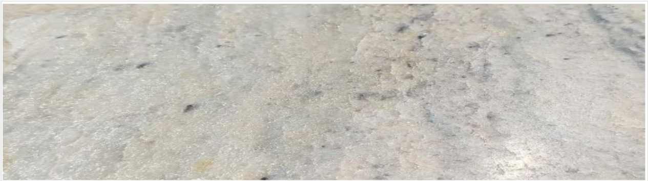
Figure 1. White Quartzite produced from test block, VMC Quarry #2
