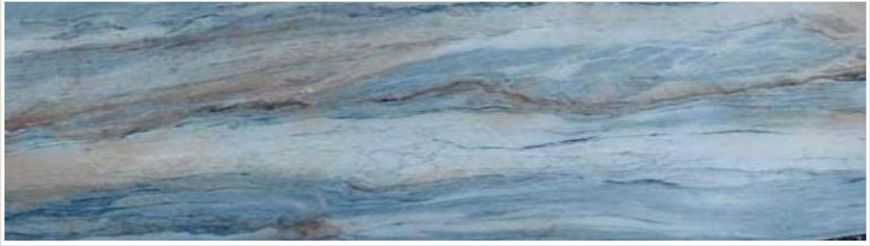
Figure 2. Blue-Grey Quartzite produced from test block, VMC Quarry #3
